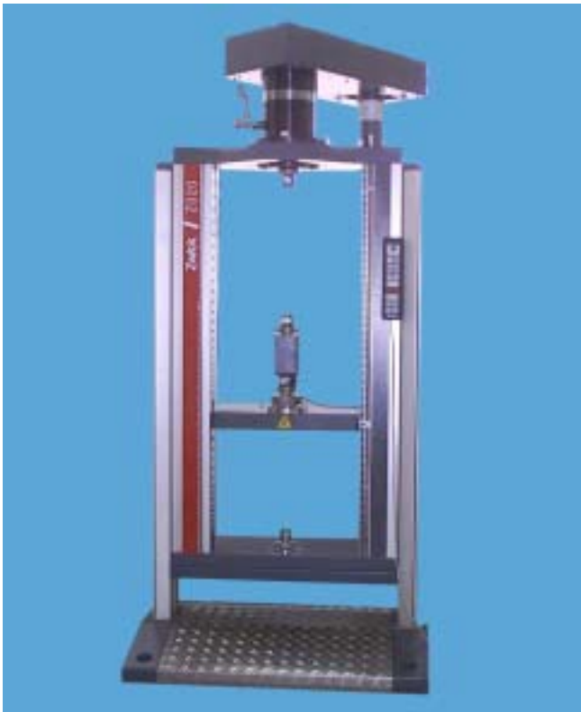
Pic 1: Zwick Z020 Materials Testing Machine with torsion drive
