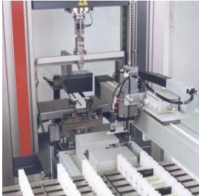
Pic 3: Feeding of a bending sample into the testing machine
