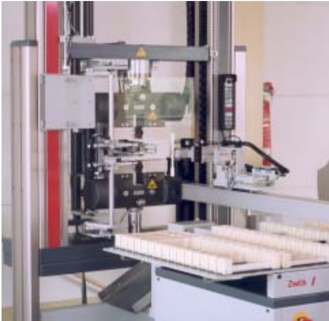
Pic 2: Feeding of a tensile sample into the testing machine
