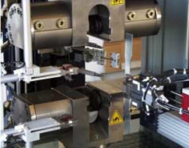
Pic 2: Feeding of the metal sample into the hydraulic grips
