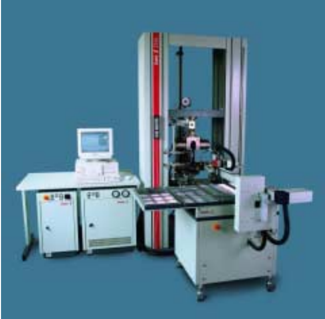
Pic 1: Automatic Specimen Feeding System „X-Linear“ for metals
