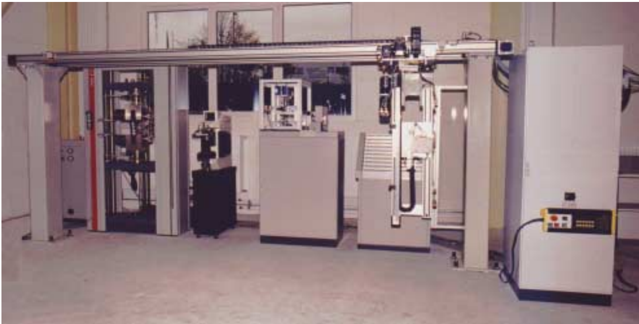
Pic 1: Automatic Specimen Feeding „Portal“ for testing of hot strip
