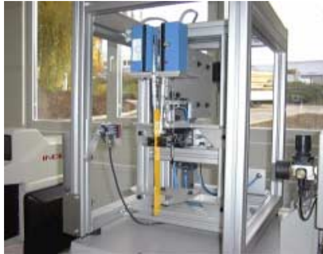
Pic 3: Roughness measuring unit and double-sided measurement
