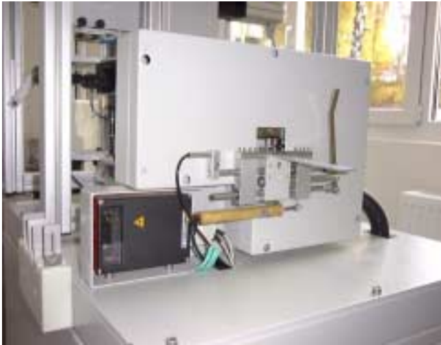
Pic 2: Cross-Section measuring and barcode-reader
