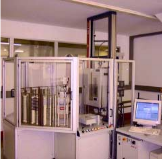
Pic 1: Automated specimen feeding system in „Polar“ construction
