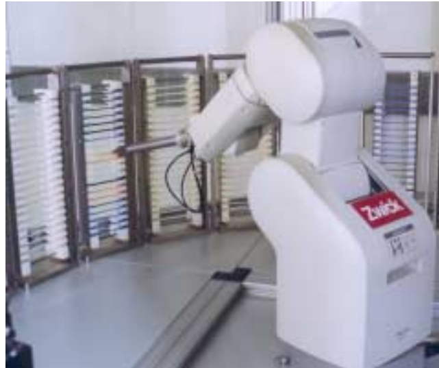
Pic 3: Taking a tensile sample out of the magazine
