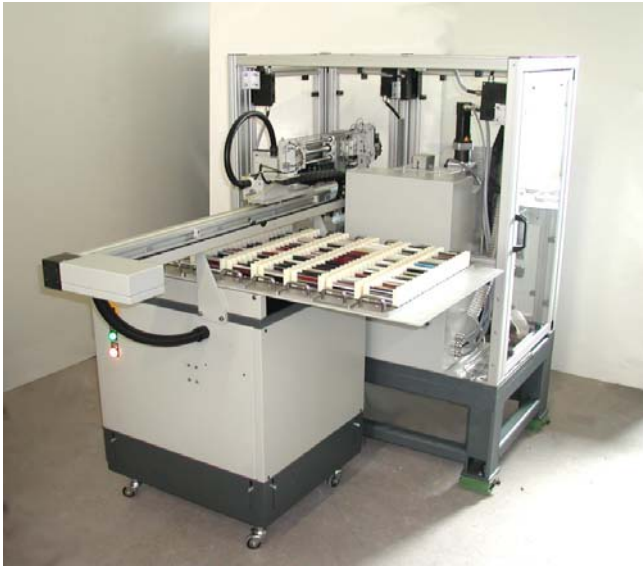
Pic 1: Complete view of the X-linear-system with notch milling machine
