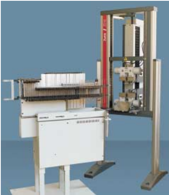
Pic 1: Automatic Specimen Feeding System „Clamp“ Type
