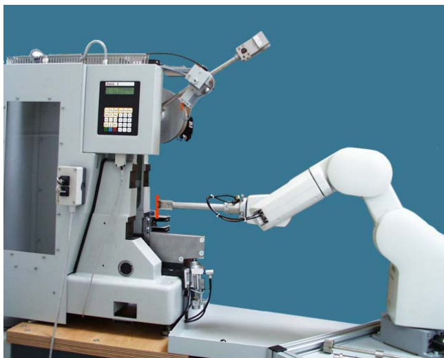
Pic 1: Automatic pendulum with a polar specimen feeding system
