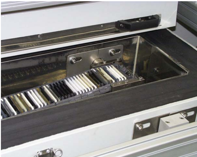
Pic 2: Specimen in the opened temperature chamber
