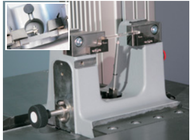
Fig. 3: Notch alignment unit at the Charpy vise
