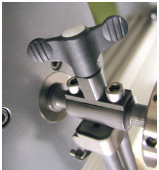
Fig. 2: Pendulum quick release for fast changing of pendulums
