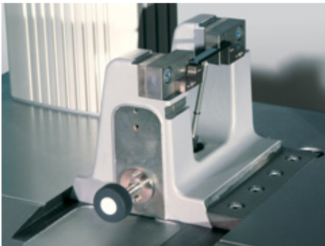
Fig. 2: Charpy vise showing large slideway area and clamping wedge
