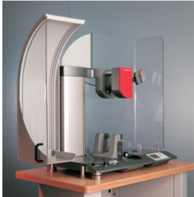
Fig 1: Pendulum Impact Tester HIT5.5P with opened safety shield
