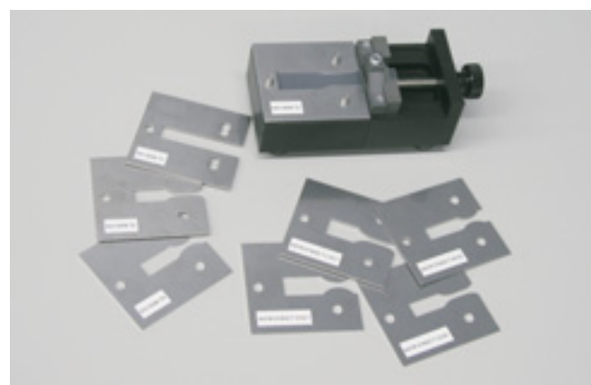
Fig. 4: Clamping gage and templates for the tensile impact test
