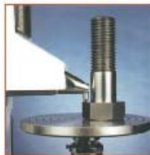
Measuring of the contact surface of a high-strength screw
