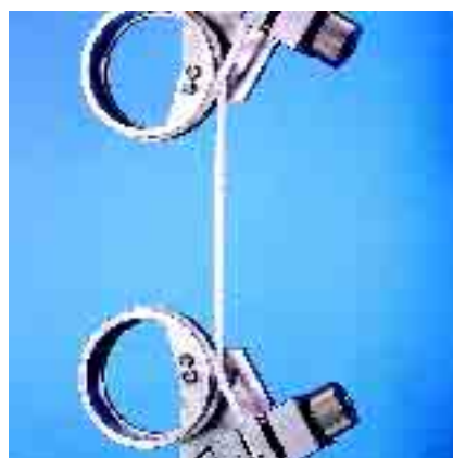
Rope grips with mechanical end clamping
