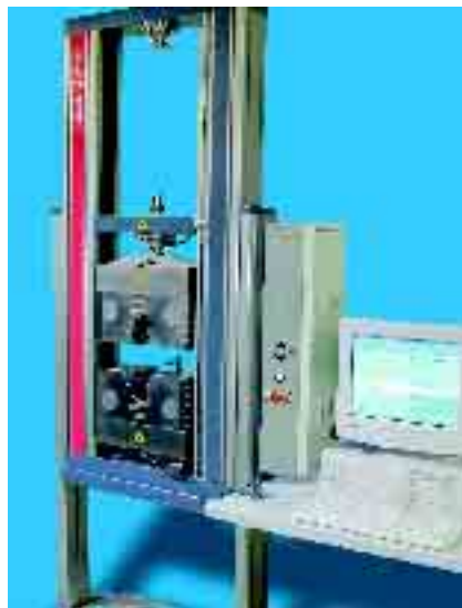
Material testing machine Z050 with testControl PC variant
