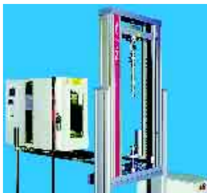
Temperature chamber mounted on guide rails
