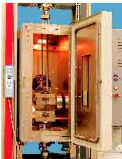
Temperature chamber with pneumatic grips (door opened)
