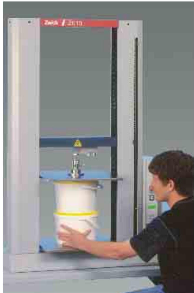
Determination of the stacking height of plastic buckets with a materials testing machine BasicLine Z010
