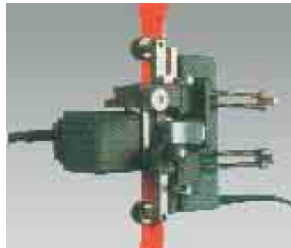
Bi-axial incremental extensometer
