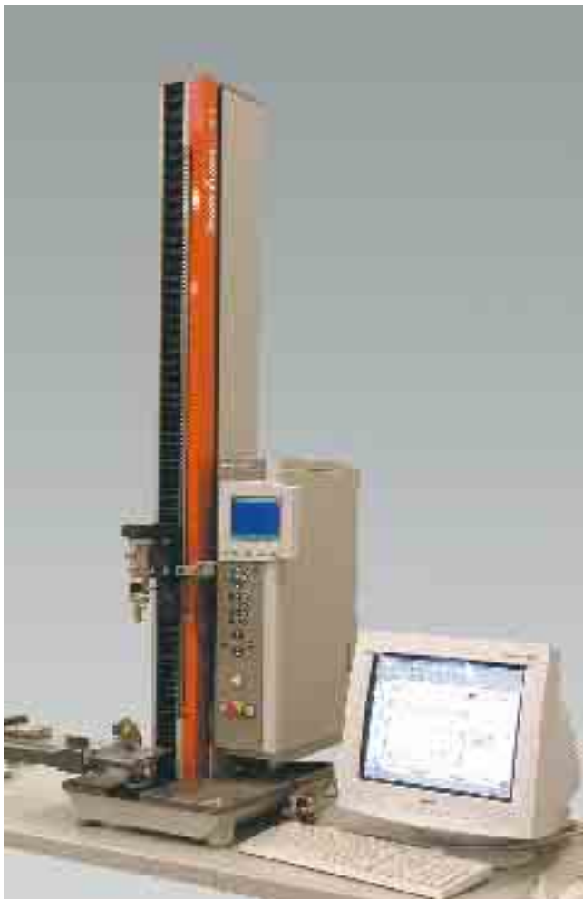
Materials testing machine zwicki Z.2.5 with test tool for the determination of the coefficient of friction on plastic films
