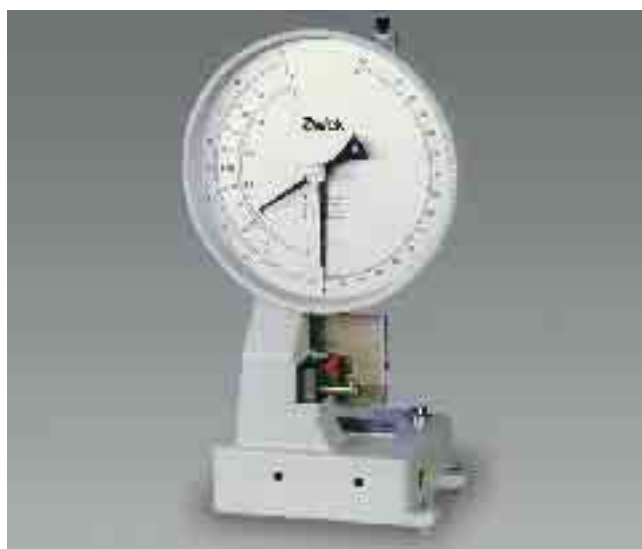
Pendulum impact tester Zwick 5102 (5 Joule) with analog display
