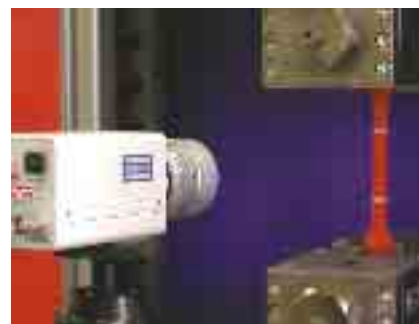
The video extensometer is adapted to the job in question by selecting suitable objectives and the object distance
