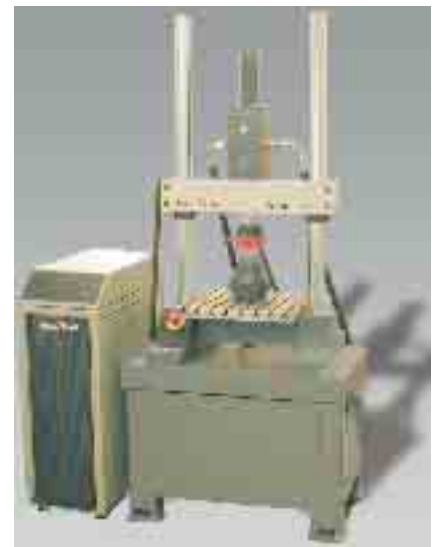
Servo-hydraulic testing machine Amsler HC 15 for testing rubber mountings
