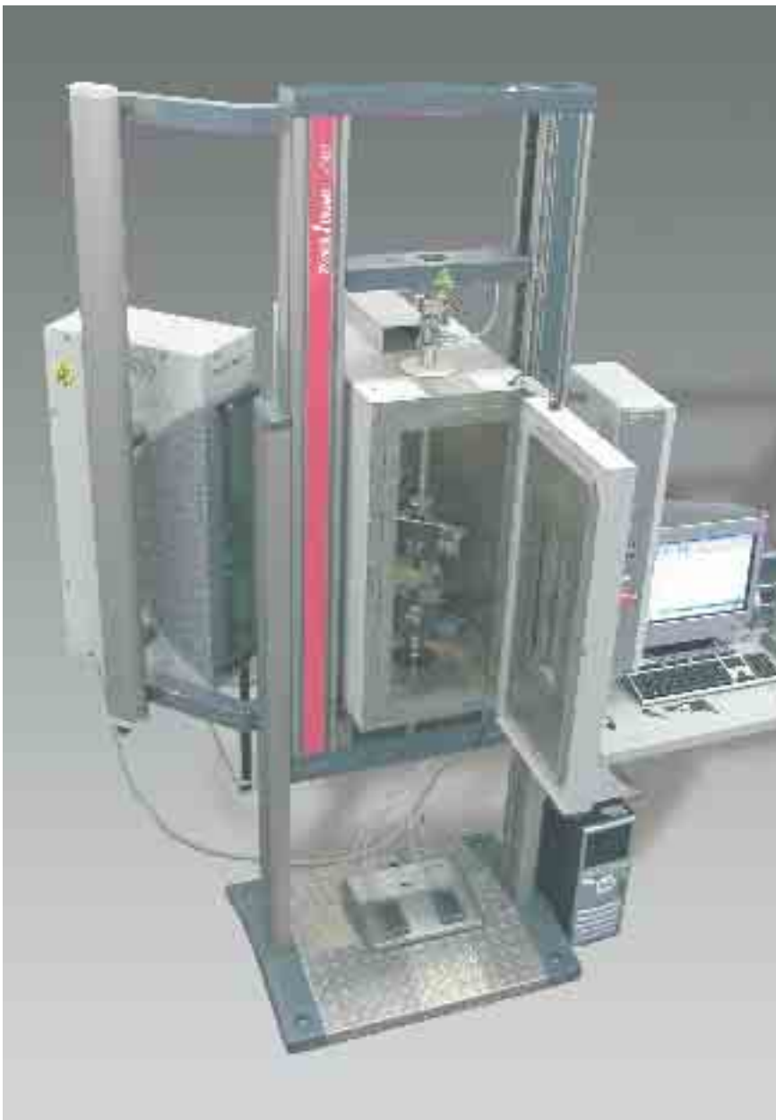
Temperature chamber, optiXtens extensometer and pneumatic grips mounted in a material testing machine Z005
