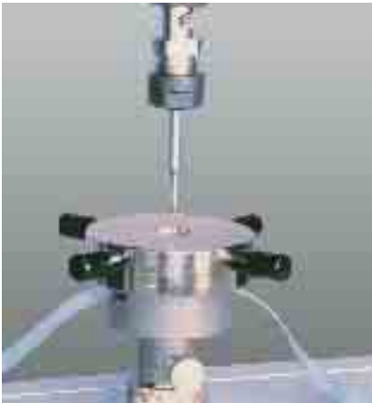
Puncture test device acc. to prEN 14477
