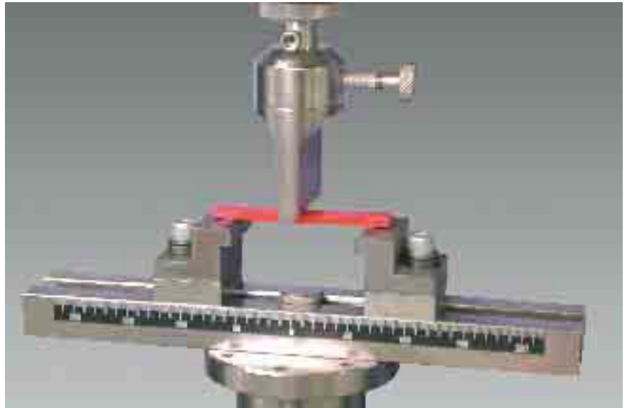
Flexural tool according to ISO 178
