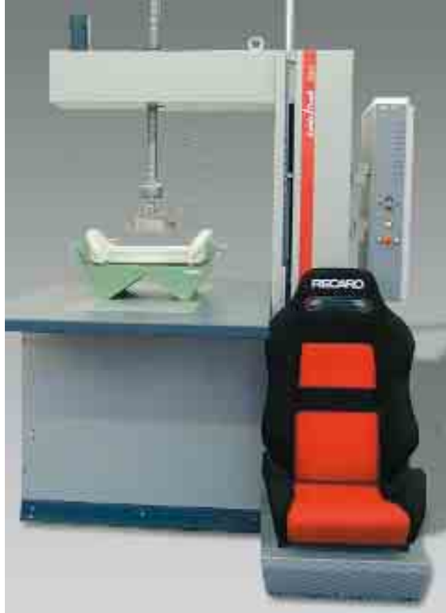
The C-shape frame is used for compression and indentation tests on larger parts of cellular plastics
