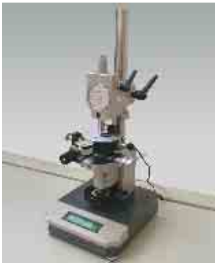
IRHD Micro Compact hardness tester 3103
