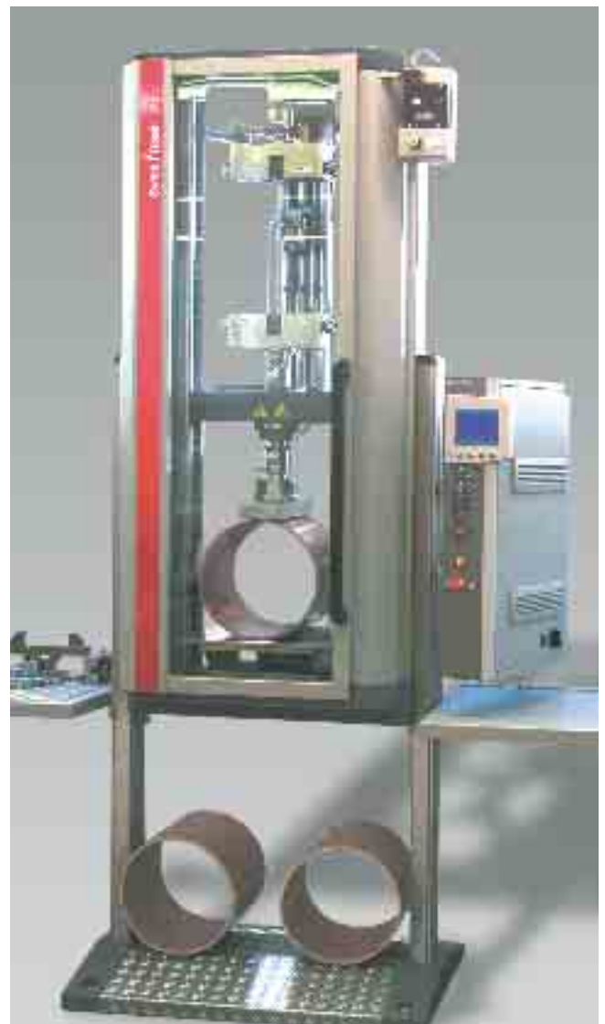
Materials testing machine Z05 in extended version for determination of tensile properties and ring stiffness of plastic pipes.
