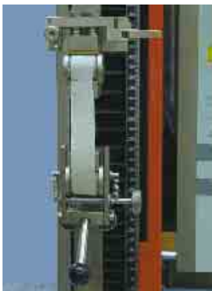
Fig. 50: Tensile test on initial wet paper
