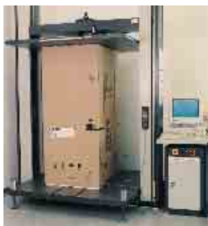
Fig. 58: Measuring the local variation deformation of a packing box
