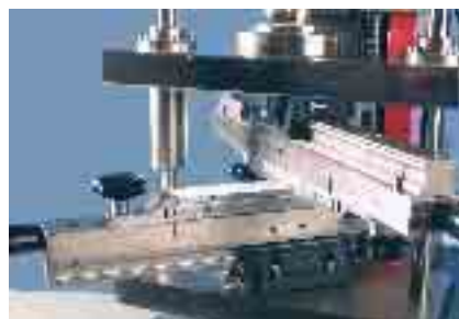
Fig. 38: Internal bond test, test run
