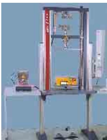
Fig. 10: Table top machine, profile legs: for tensile, burst and box crush test
