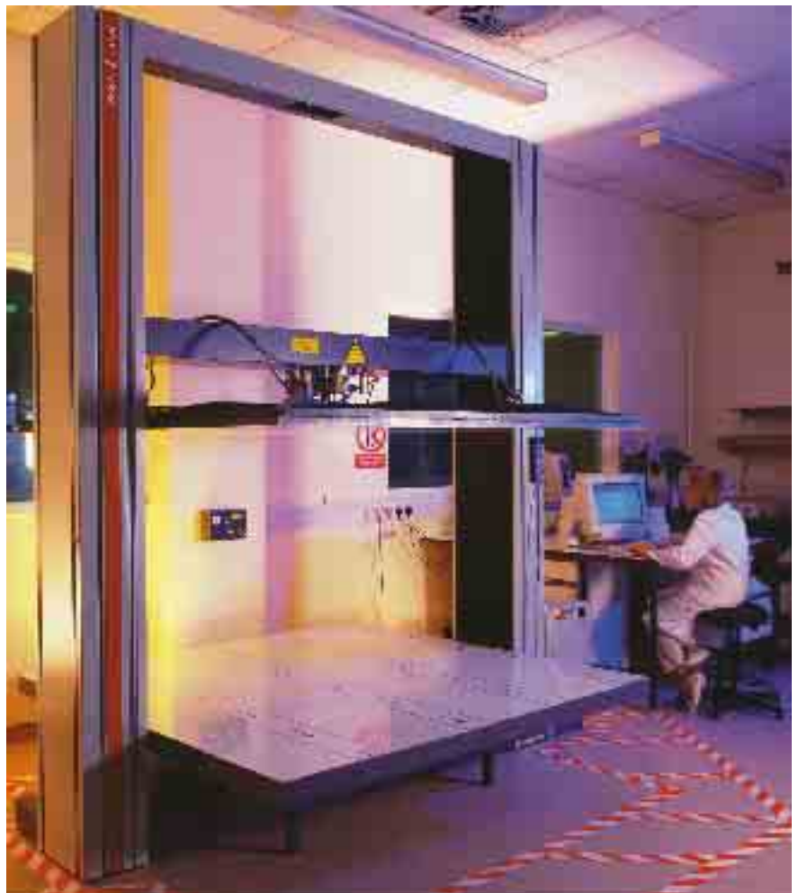
Fig. 44: Box-crush tester for specimen up to a footprint of 2 m by 2 m (authorized by SCA Packaging Research, European Technical Centre, Aylesford)
