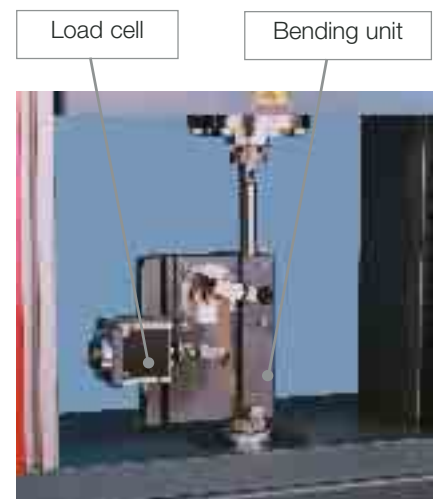
Fig. 17: 2-Point bending unit, set-up
