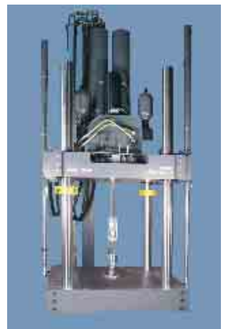
Fig 62: High speed testing machine, up to 20 m/s
