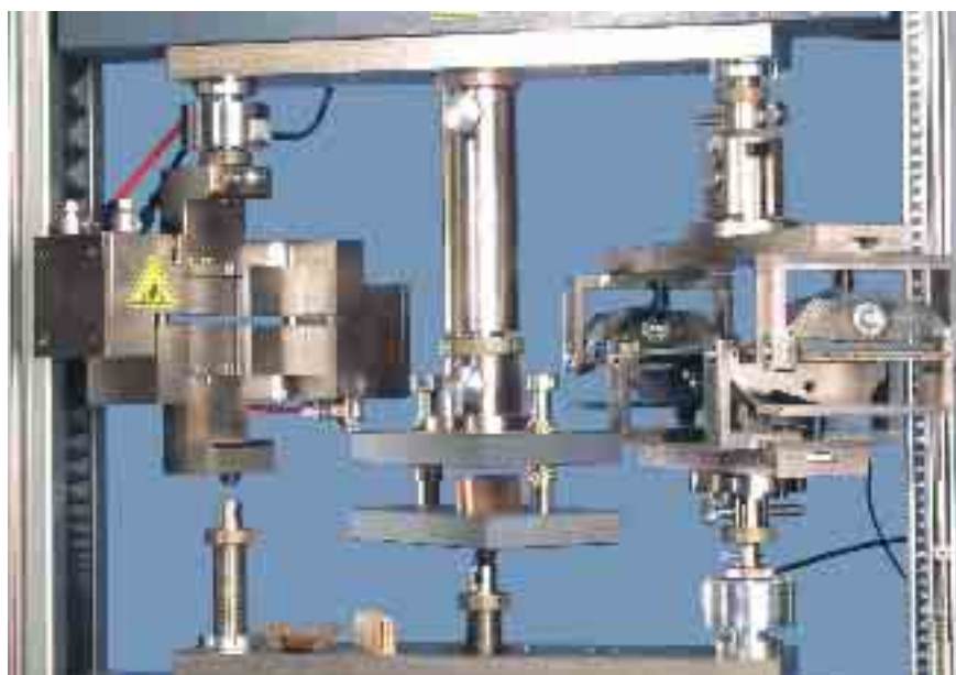
Fig. 7: Materials testing machine for all tests to predict the box's strength
