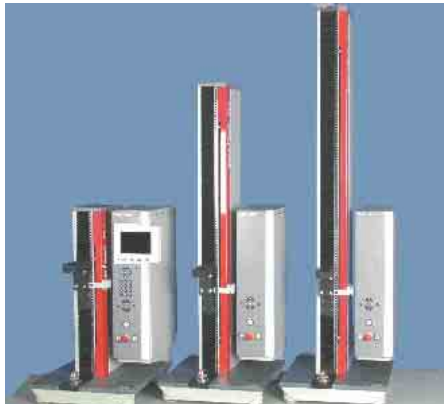
Fig. 9: 2.5 kN zwicki testing machines: testControl stand alone version (left), PC variant (mid and right)
