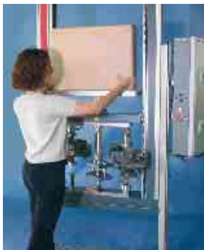
Fig. 6: Accessories for strip crush, edge crush and flexural tests
