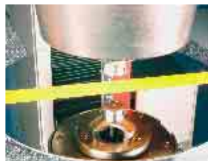
Fig. 59: Compressibility test head prior to test
