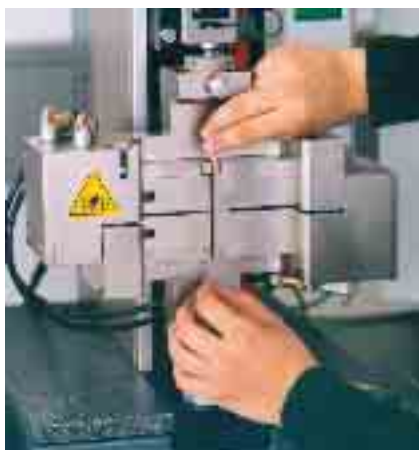
Fig. 34: Strip crush test grips
