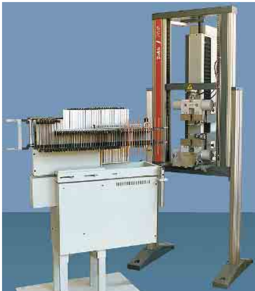
Fig. 63: Automatic testing machine: tests on sanitary products
