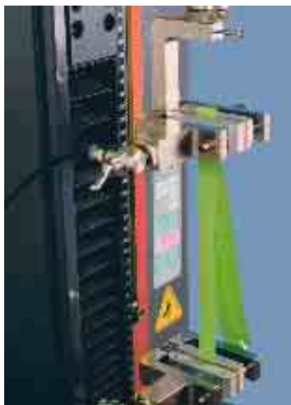
Fig. 51: Tensile test on dry paper, pneumatic specimen grips
