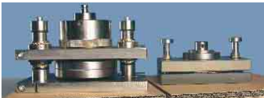
Fig. 32: Compression plates for the flat crush test on miniature corrugated board (left, F > 10 kN) and on standard corrugated board (right, F \leq 10 kN)
