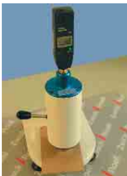
Fig. 23: Thickness gauge for corrugated board
