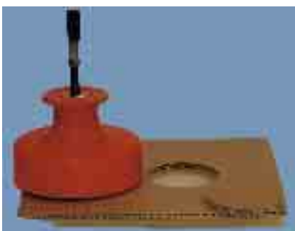
Fig. 52: Circular cutter for FCT specimen
