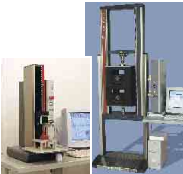
Picture 41a/b: Testing machines of the Standard series: A 1-column (left) and 2-column (right) table-top machine
