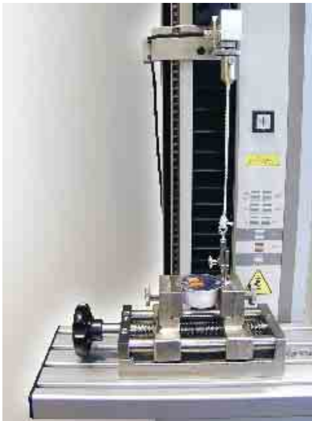
Picture 39: Pull-off test on a marmalade container which is held in a parallel vice. The pull-off is performed by a small screw clamp
