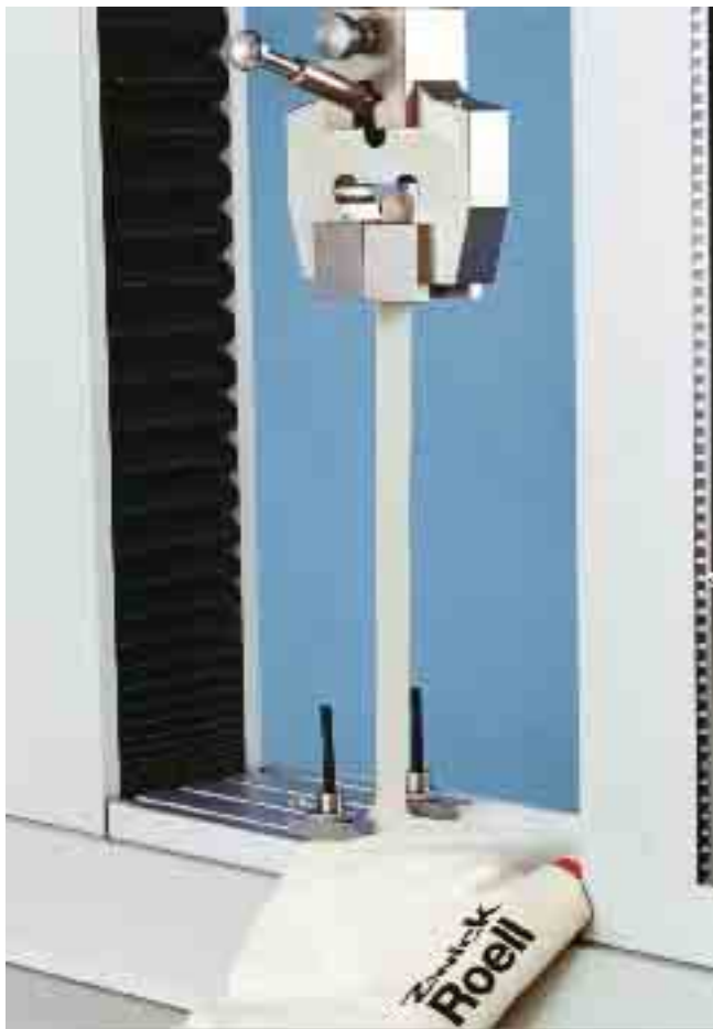
Picture 50: An individually specified test arrangement: Above is a specimen grip and below are elements of the BasicLine Toolbox
