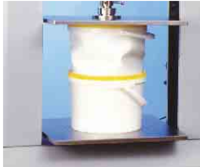
Picture 24: Stacking test on plastic pails
