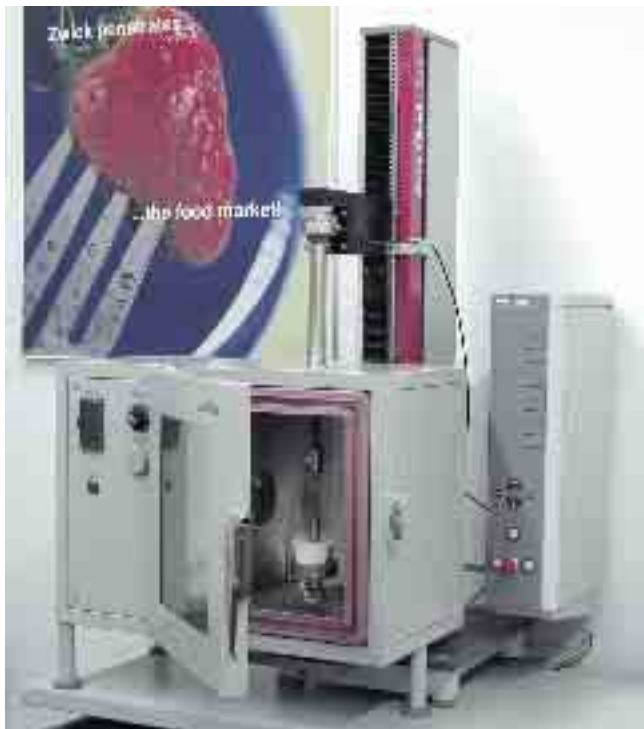
Picture 52: A temperature chamber especially for the zwicki. Used here for testing on foodstuffs
