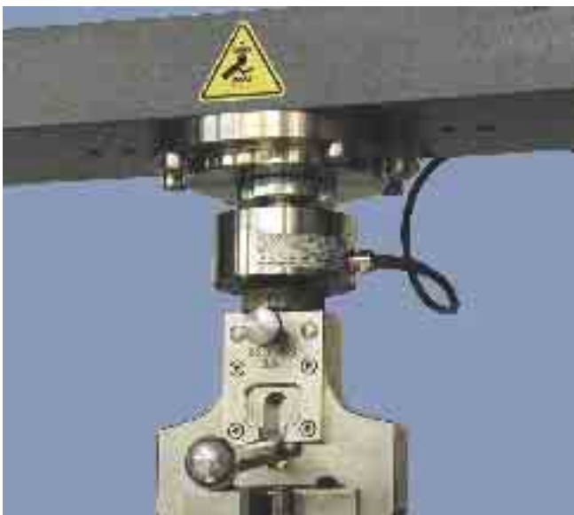
Picture 49: A load cell from our large selection: The load cell type „KAF“ for loads up to maximum 5 kN
