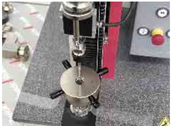
Picture 29: Penetration test on foil strips
