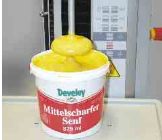
Picture 5: Viscosity test on mustard
