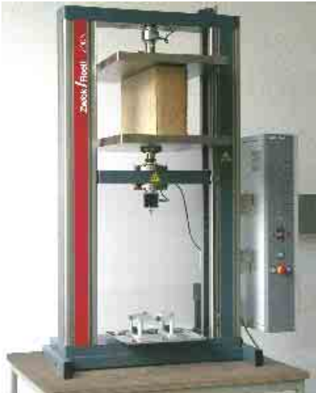
Picture 44: By equipping a testing machine with several testing positions, a maximum degree of use is achieved at low cost
