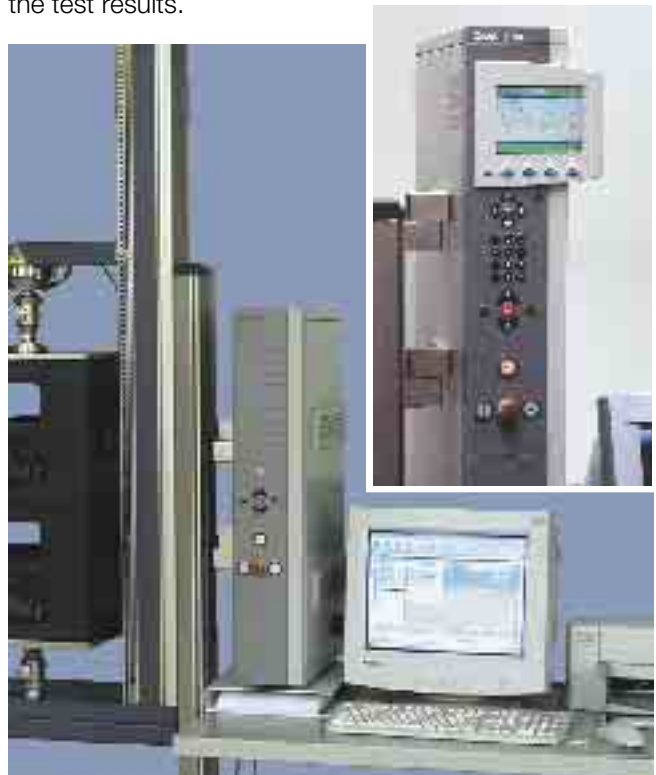
Picture 47: The measurement, control and regulating system testControl is operated via PC, or with the option „Stand Alone“ also without PC (see inset picture)
