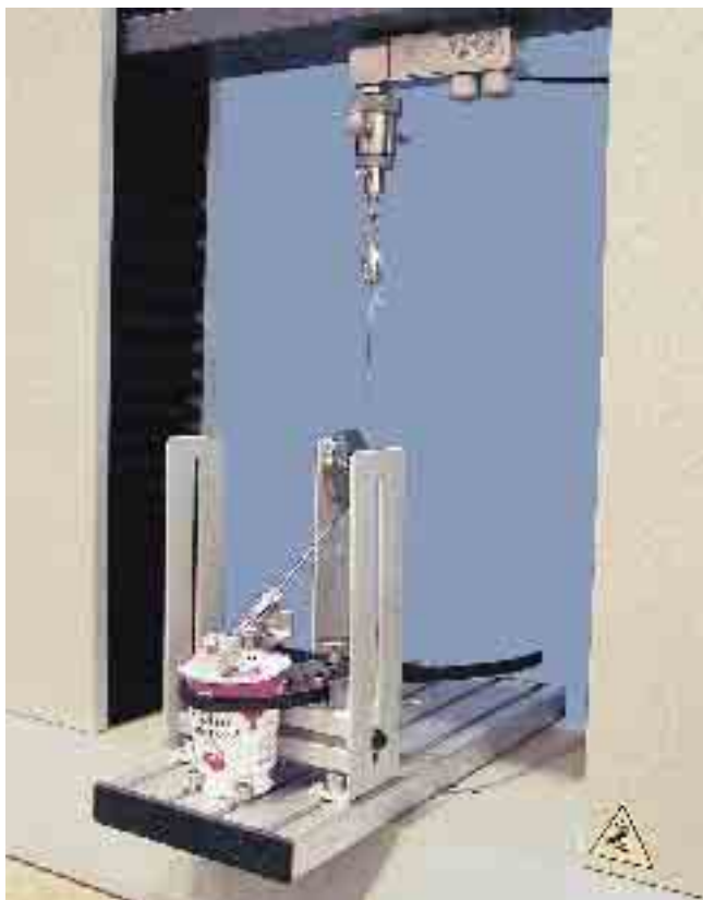
Picture 35: Peel-off test on a packaging beaker
