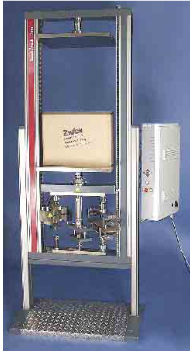
Picture 51: The „Mc Kee-testing machine“ contains the most varying testing units especially for packaging / paper testing
