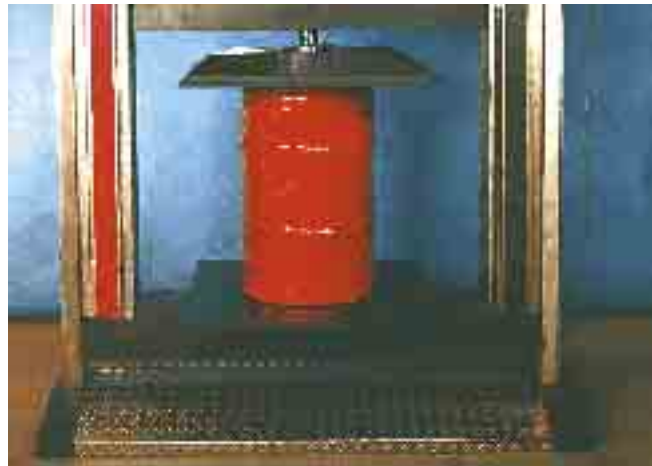
Picture 34: Compression test on a metal barrel
