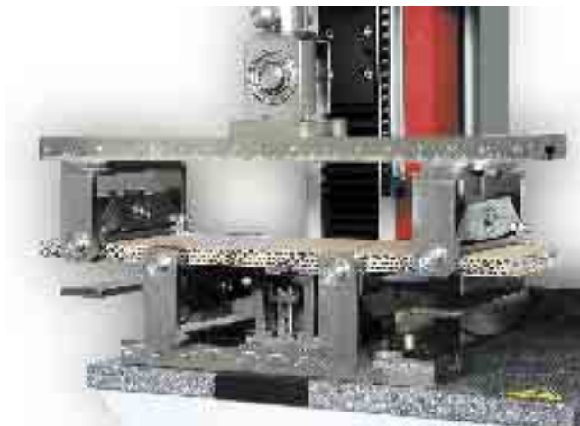
Picture 32: 4-point flexure test on cardboard
