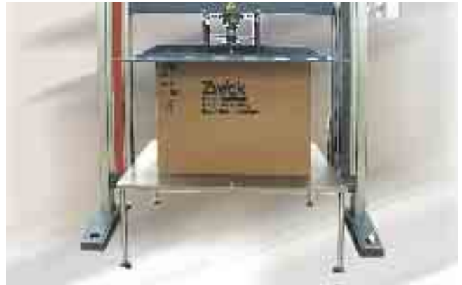
Picture 31: Box compression test on a large cardboard box
