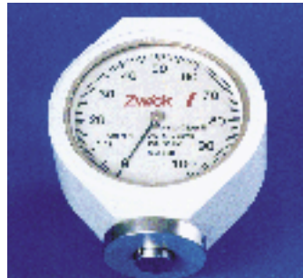
Picture 20: Sausage hardness testing with a Shore A hardness tester
