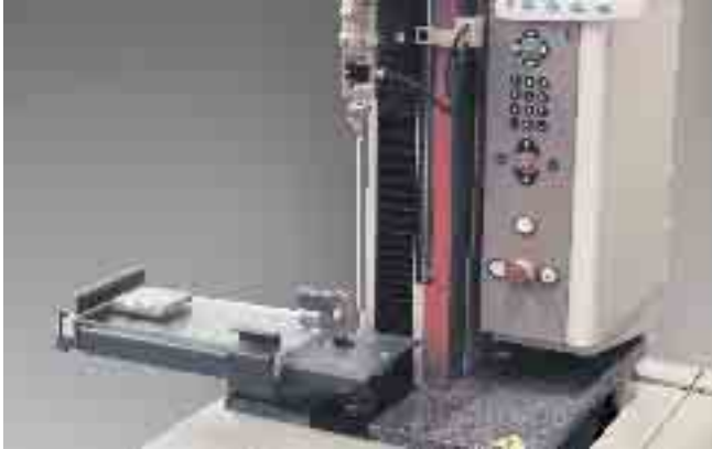
Picture 28: The device for testing the frictional behaviour, mounted
