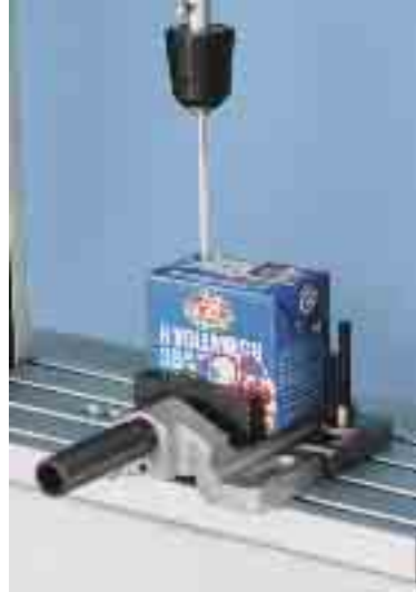
Picture 40a/b: Penetration tests on foodstuffs packaging
