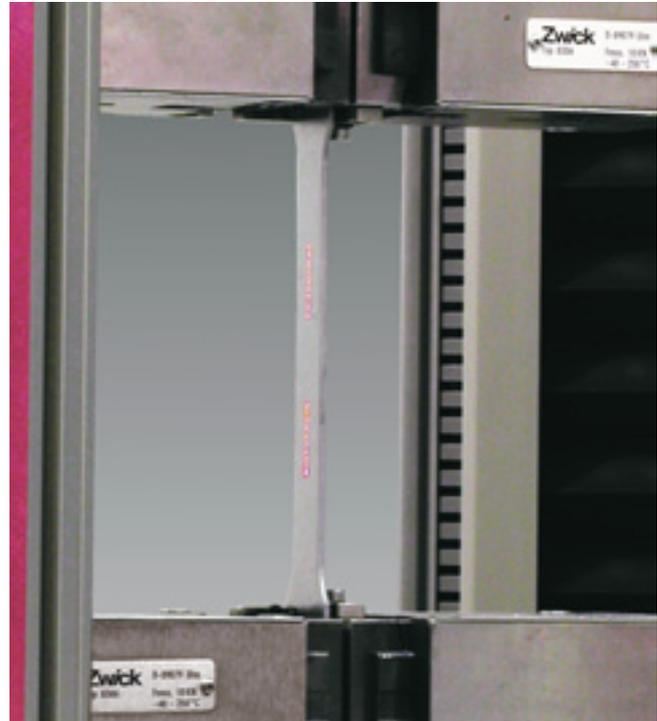
Fig. 31: The line lighting of the specimen surface with coherent laser light.
