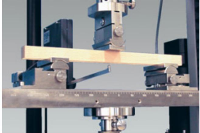
Fig. 20: Extensometer for 3-point flexure test
