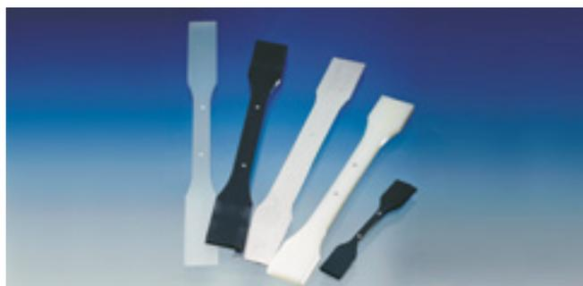
Fig. 22: Marked specimen for optical measurement
