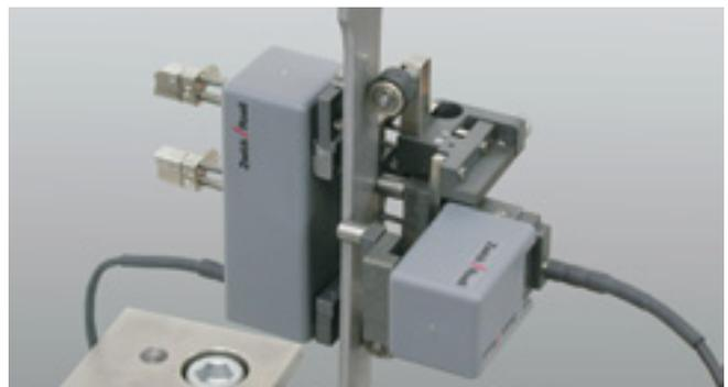
Fig. 16: Biaxial incremental clip-on extensometer
