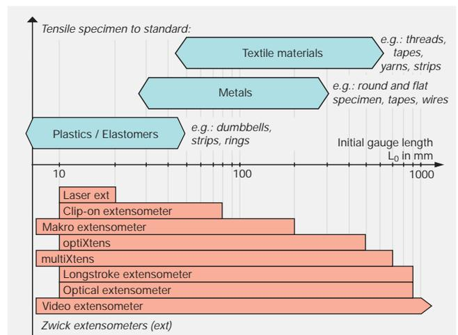
Diagram 2: Application range of Zwick extensometers dependent upon the initial gauge length  $L_0$
