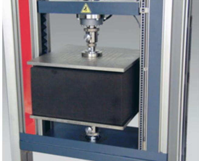
Fig. 2: The extension is measured indirectly at this compression test
