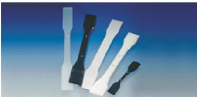
Fig. 22: Marked specimen for optical measurement
