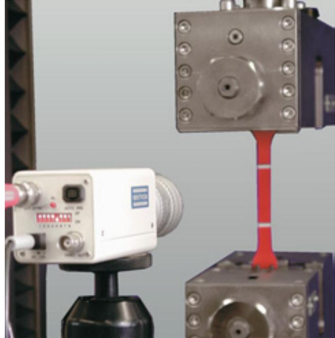
Fig. 27: The specimen surface is digitalised by a full-frame camera
