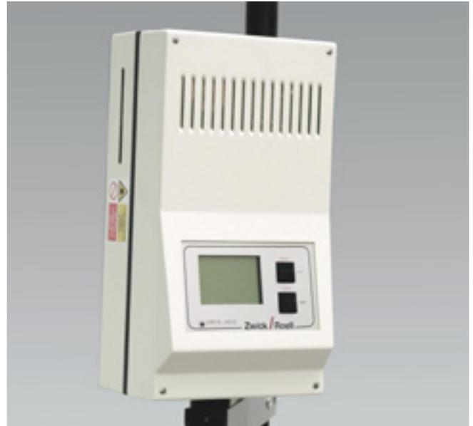
Fig. 25: The laser extensometer, here separated from a test system
