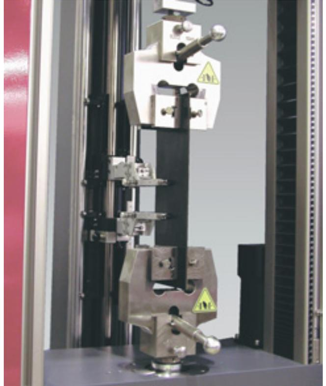
Fig. 11: Longstroke extensometer
