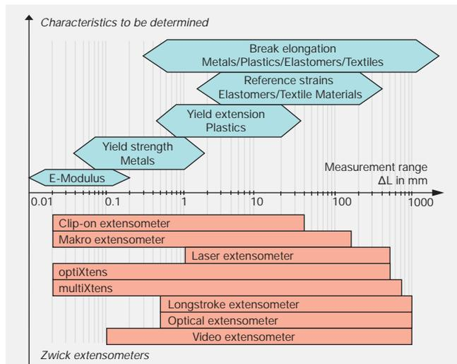
Diagram 3: Range of application of Zwick extensometers dependent upon the measurement travel
