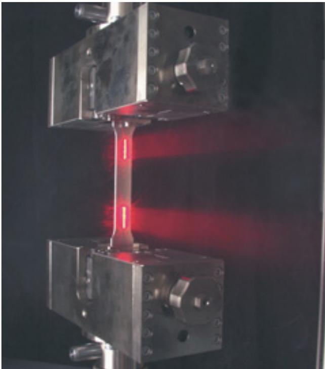
Fig. 21: A technology only offered by Zwick: Testing with optiXtens
