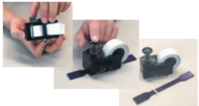
Fig. 26: The specimen marking devices are simple to operate and are functionally safe (Here a simple manual device)
