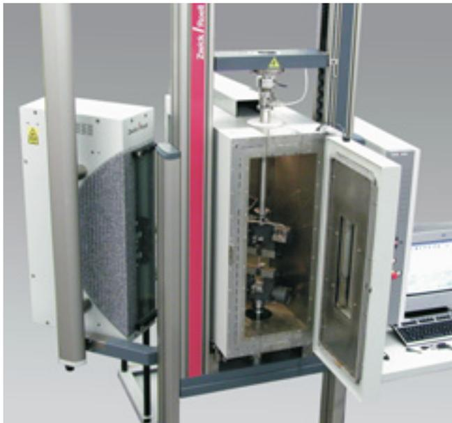
Fig. 30: optiXtens in conjunction with a temperature chamber
