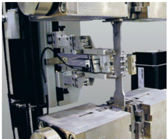
Fig. 10: Macro extensometer in combination with a reduction in width monitor (With 4 measurement lines)
