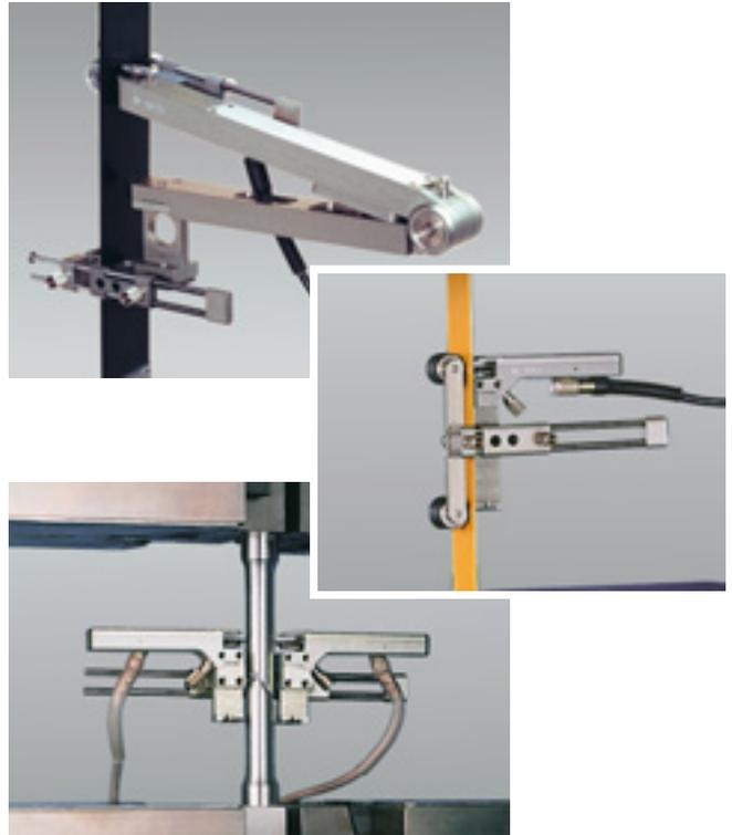
Fig. 19: Strain gauge clip-on extensometers
