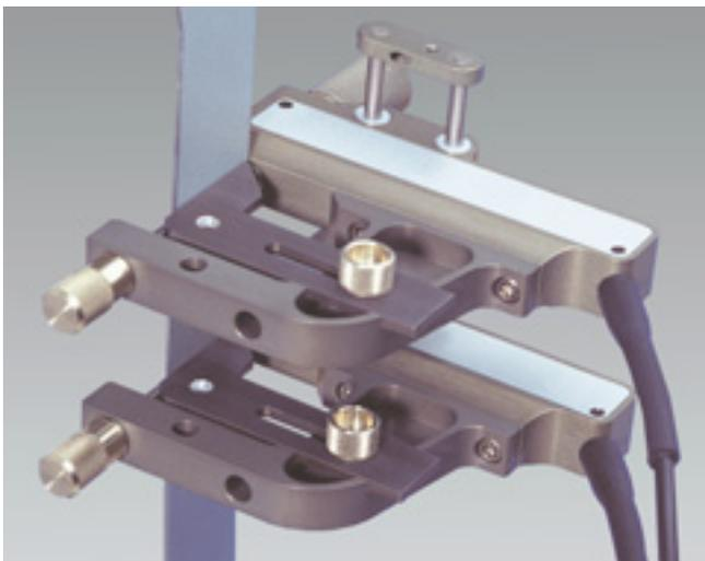
Fig. 18: Strain gauge clip-on extensometer for width measurement
