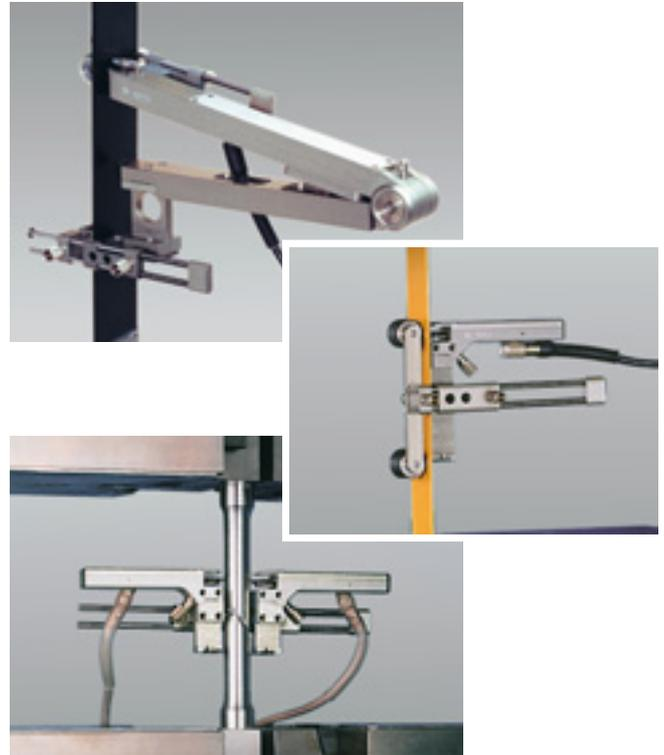
Fig. 19: Strain gauge clip-on extensometers
