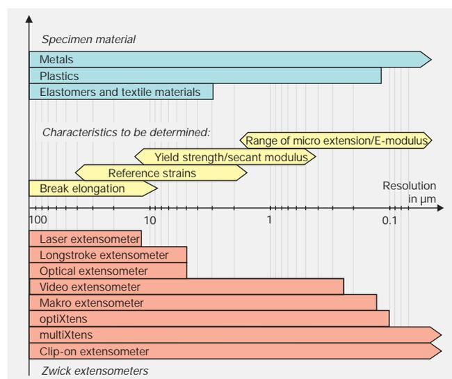
Diagram 1: Range of application of Zwick extensometers dependent upon the test data resolution
