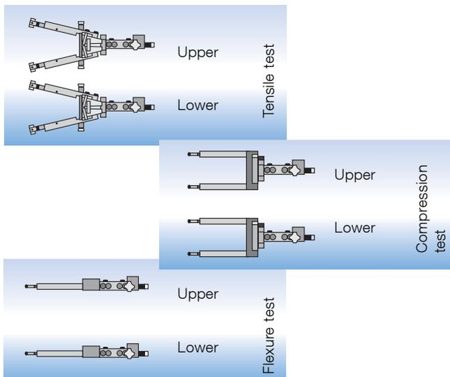
Fig. 4: Different types of sensor arm increase the range of application
