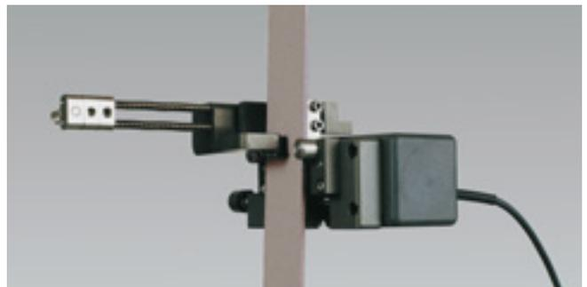
Fig. 15: Incremental reduction-in-width monitor
