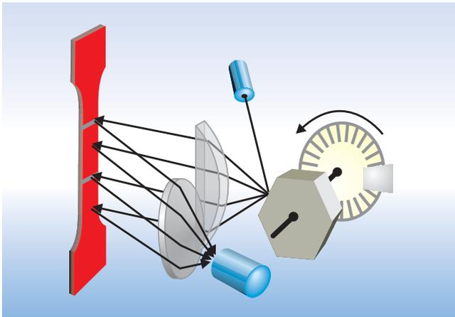
Fig. 24: The principle of the laser extensometers
