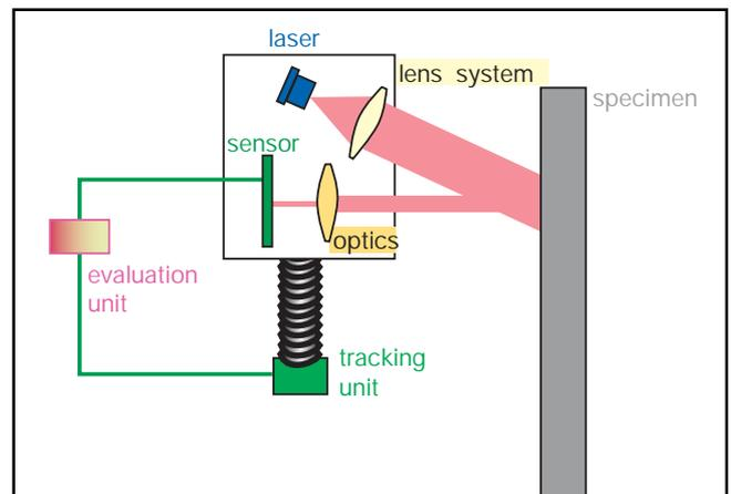
Fig. 29: optiXtens (Upper measurement head) setup and principle of tracking the reference speckle
