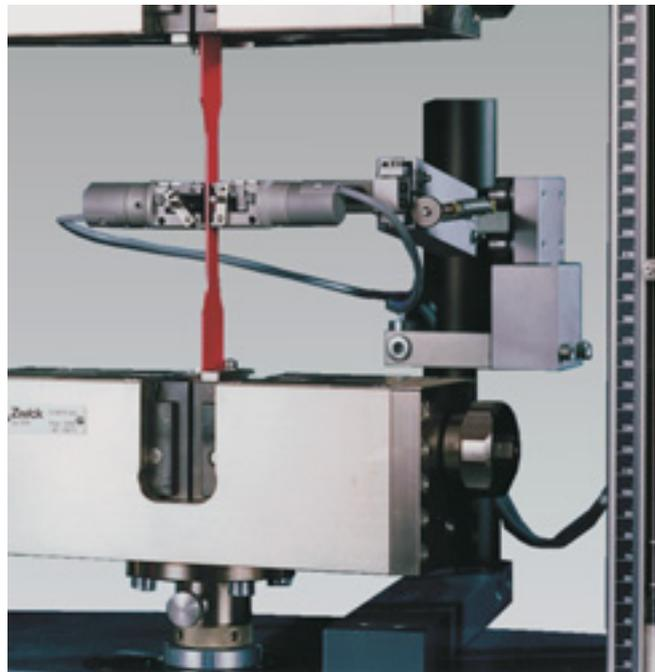
Fig. 17: Analogue clip-on extensometer 066251 with optional counter weight system
