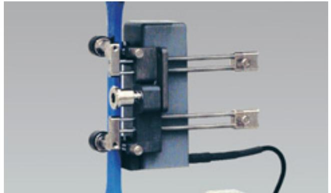
Fig. 14: Incremental clip-on extensometer (TC-EXICLEL.002)
