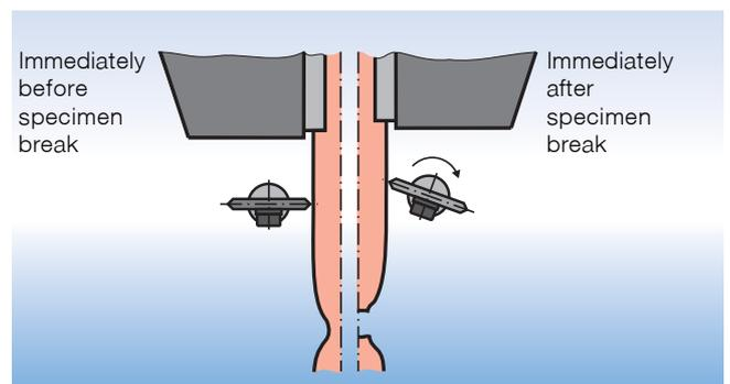
Fig. 6: Principle function of the tiltable knife edges
