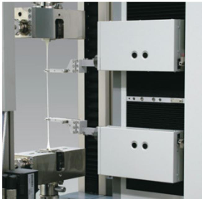
Fig. 7: The measurement heads were mounted on the measurement carriages. The easy to change sensor arms get fixed on the measurement heads.
