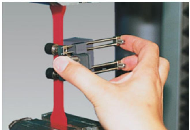
Fig. 12: The incremental clip-on extensometer guarantees simple and rapid handling.
