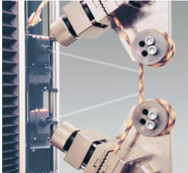
Fig. 23: The optical extensometer for non-contact measurement
