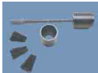
Specimens of reinforcement bars with clamping jaws
