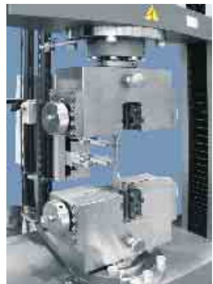
Wedge screw grips 8506 (100 kN)
