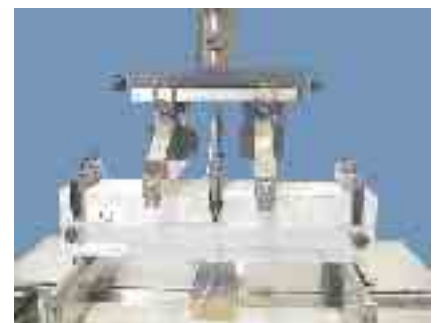
Transducer for measuring the bending deformation
