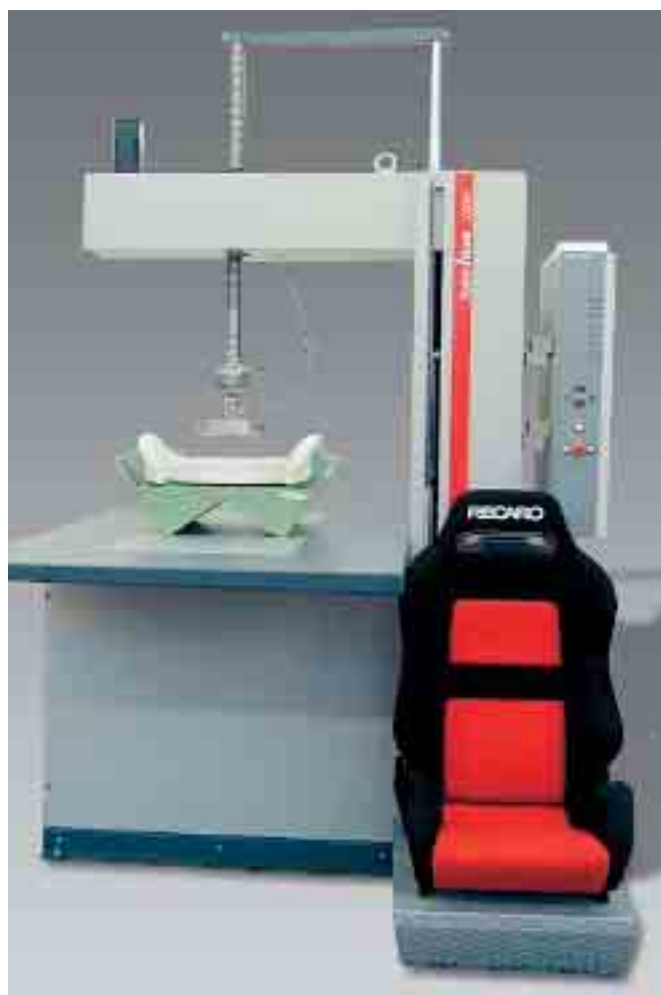
The C-shape frame is used for compression and indentation tests on larger parts of cellular plastics
