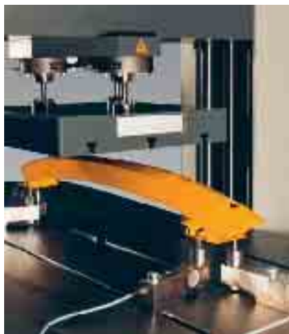
Buckling strength test system for bumpers
