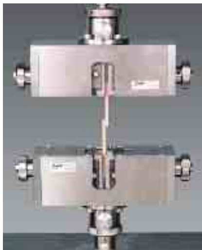
Tensile test of welded lap joint using special synchronized mechanical grips
