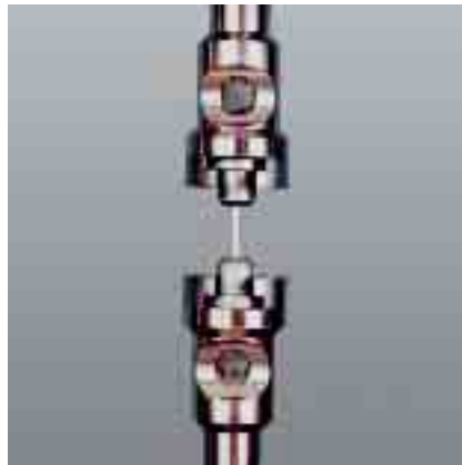
Tensile test on Fasteners
