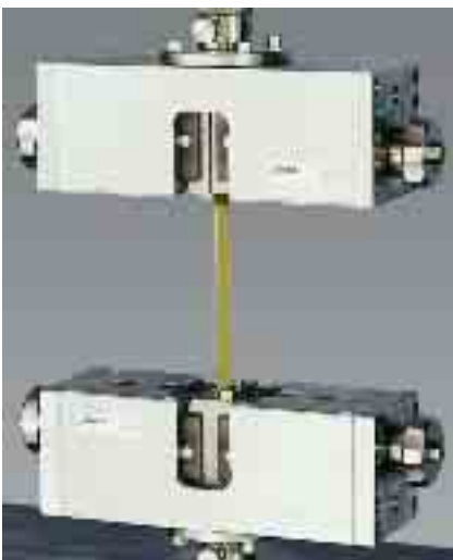
Tensile test of welded specimen
