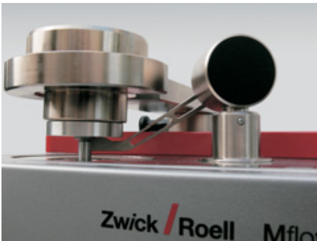
Mflow: its extensometer measures with high precision
