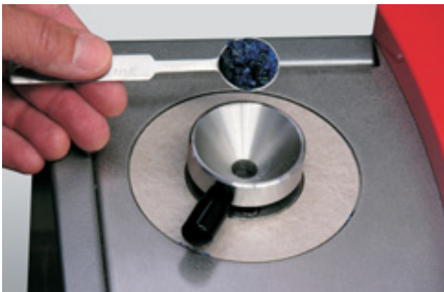
Easy filling of the barrel with the portioning gage
