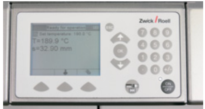
The clearly arranged control panel indicates all parameters and test results
