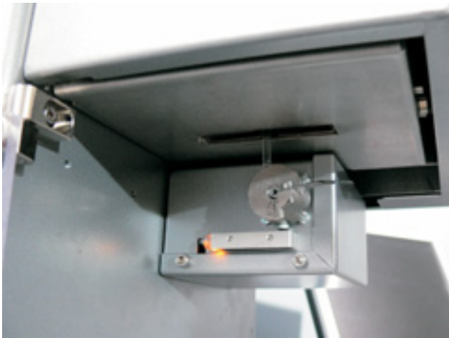
Extrudate cutter, operated automatically
