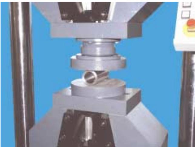
Fig. 16: Compression platens for performing compression tests
