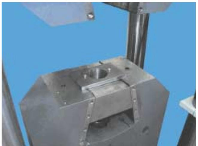
Fig. 18: Calibration mounting for SP Machine
