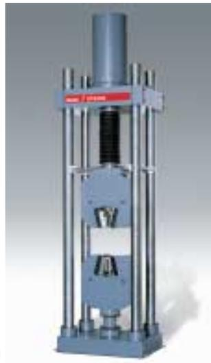
Fig. 02: Zwick SP2000 load frame; 4 columns, adjustable crosshead
