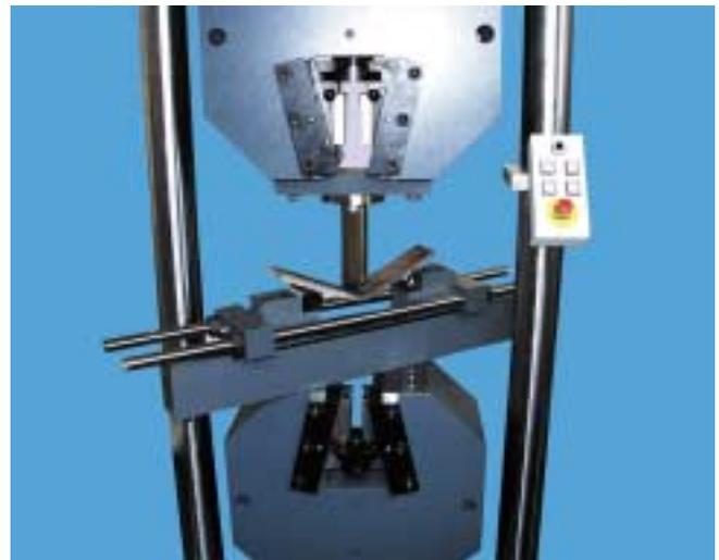
Fig. 17: Zwick SP400 with unit for performing bending tests
