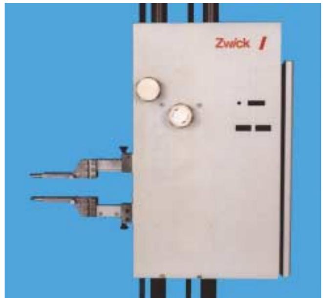
Fig. 10: Zwick extensometer Macro for SP Machine (BSP066551.02)
